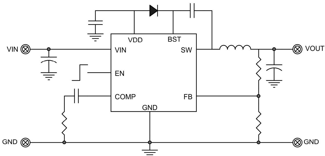
Note: When using a solid or ceramic input Cap, It is recommended to parallel a TVS diode.
